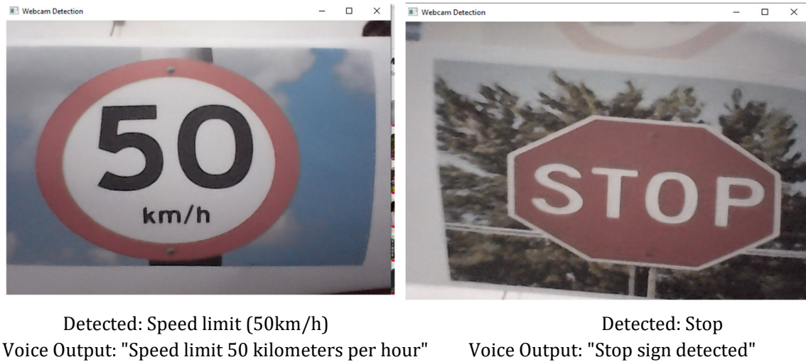
Figure 3 & 4: Real-Time Traffic signs detection
